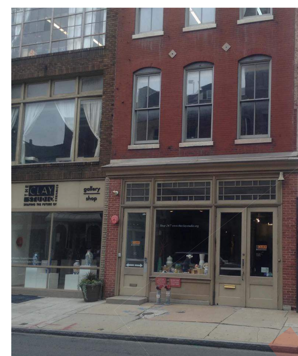
Transparent ground floor; smaller punched openings for decreased transparency in floors above to balance privacy and views
